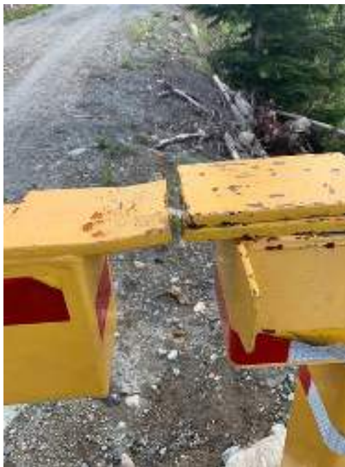
Figure 33. Vandalism of the gate (cut through with a grinder) across the Boulder Creek HEF access road documented by Project operators on May 22, 2020.
