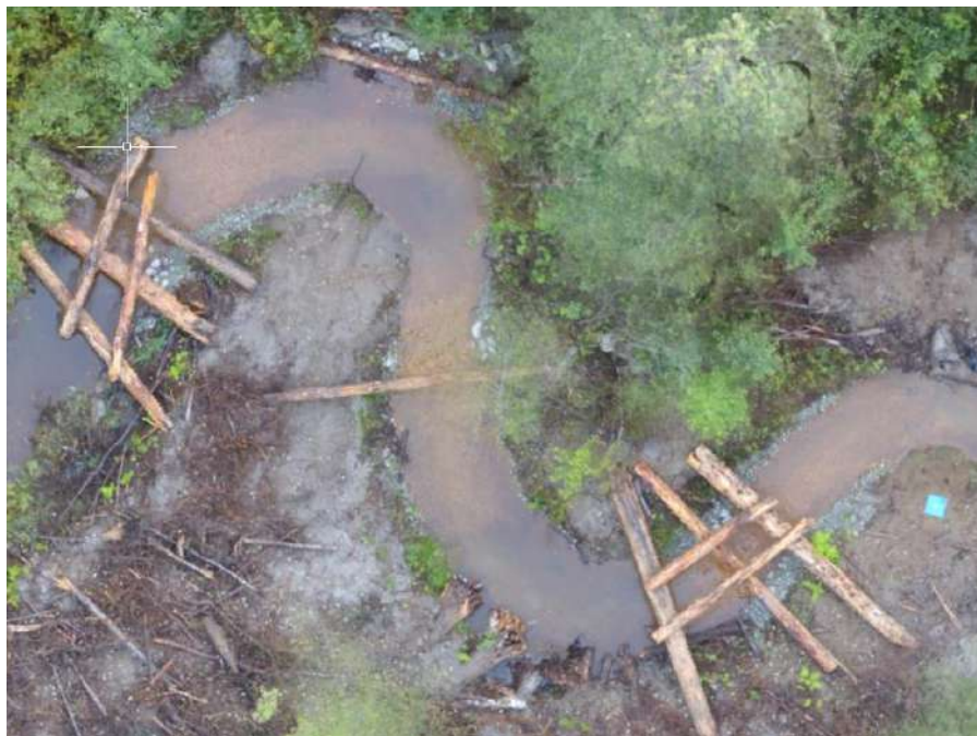
Figure 9. Sample screenshot from downstream (Reach 1) orthomosaic image showing riffle-pool sequence and habitat features for the Alena Creek FHEP.
