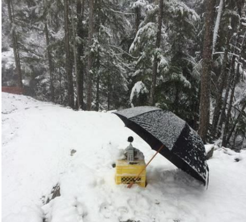
Photo 20 – Monitoring noise levels at the BDRHEF intake (November 20, 2016).
