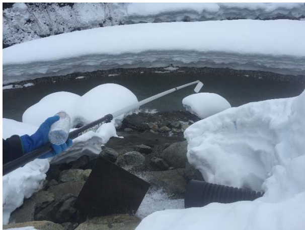
Photo 7 – Sampling discharge from ULRHEF sediment basins to Lillooet River during grouting in the tunnel (February 14, 2016).
