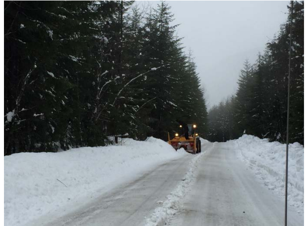
Photo 2 – Snow blower removing snow at KM33 of the Lillooet River FSR (January 19, 2016).
