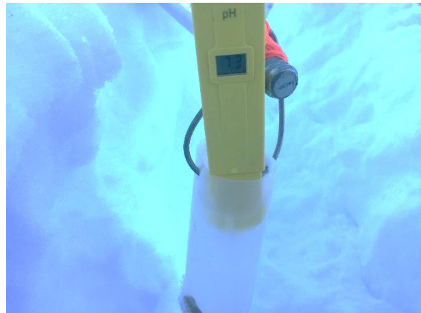
Photo 4 – pH sampling at the compliance point downstream of the ULRHEF intake sediment basins outlet (November 28, 2015).
