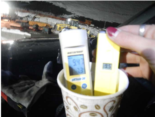
Photo 11 – pH sampling at ULRHEF intake sediment basins following grouting in tunnel (November 8, 2015).
