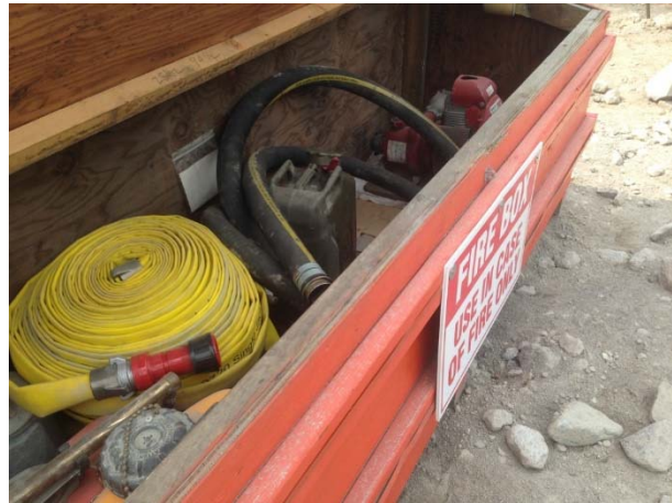
Photo 2 – Fire suppression supplies stored at the ULRHEF intake site (June 18, 2015).
