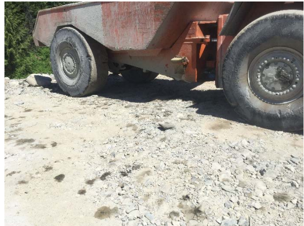
Photo 19 – Oil spotting at BDRHEF downstream portal parking area (June 8, 2015).
