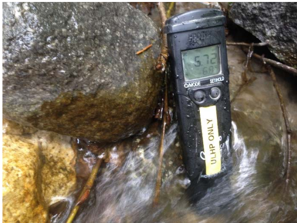
Photo 18 – ULRHEF powerhouse clear discharge to the Lillooet River during the concrete pour, pH = 6.72 (May 26, 2015).
