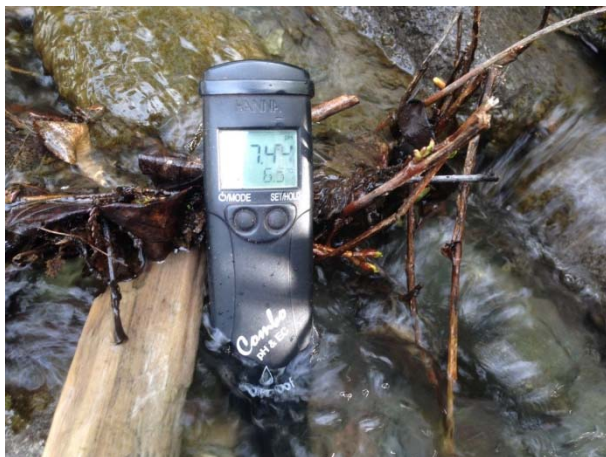
Photo 19 – pH measurement conducted at discharge point of powerhouse sump dewatering hose (May 10, 2015).
