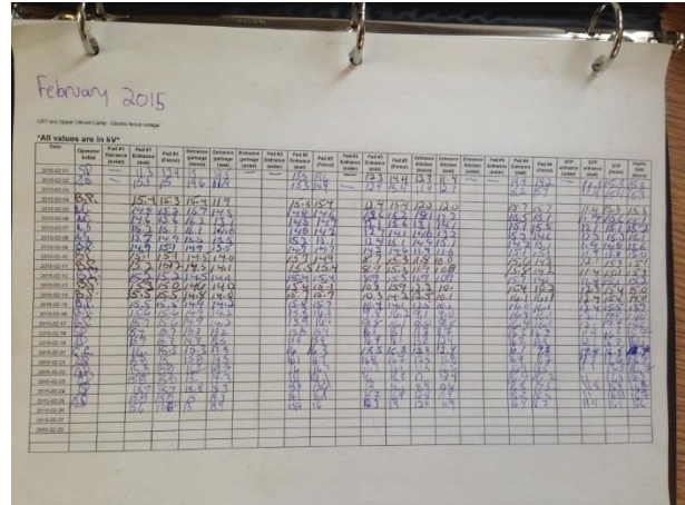
Photo 6 – Daily inspection log of the electric fence was up to date with voltages recorded during each inspection (February 26, 2015).
