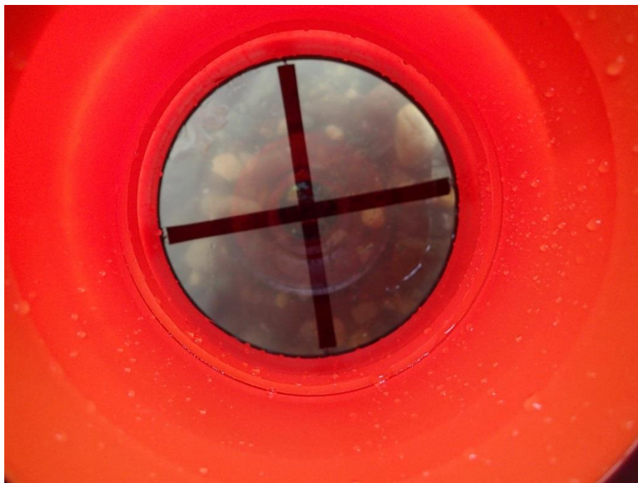
Figure 41. DSSM03 – Representative image through bathyscope viewer: after works. Rainfall-induced natural background turbidity event in the river impaired survey (November 27, 2014).
