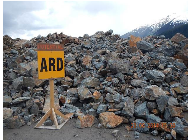
Photo 6. PAG stockpile at Truckwash Creek west heading (June 20, 2014).
