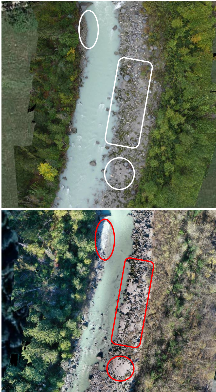
Figure 6. Upper Lillooet River Diversion Reach displaying fine sediment accumulation from 2016 (top) to 2023 (bottom).
