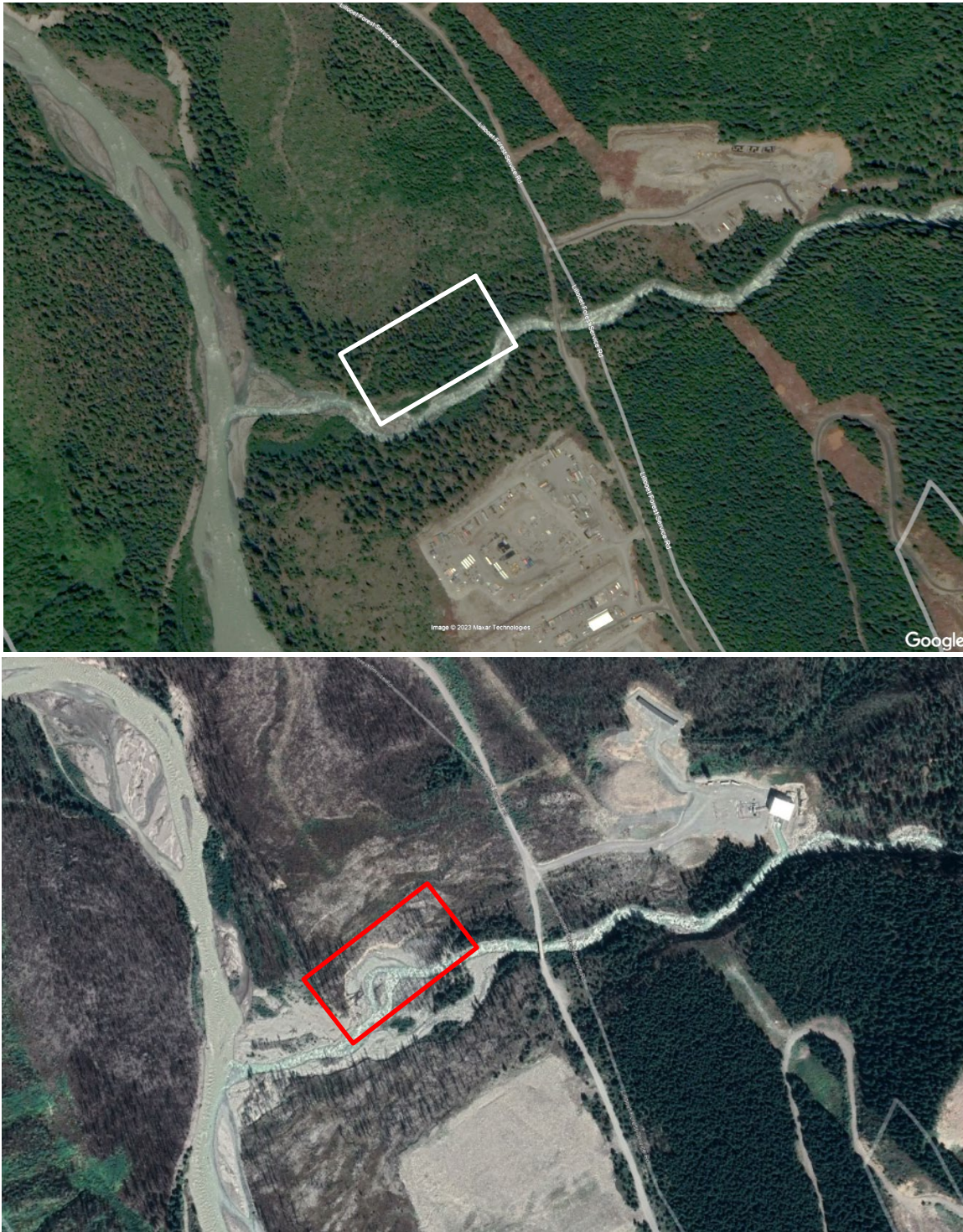
Figure 18. Boulder Creek Downstream Reach Google Earth imagery displaying the shifting of the active channel outline in red from river left to a new river right channel from 2014 (top) to 2022 (bottom).
