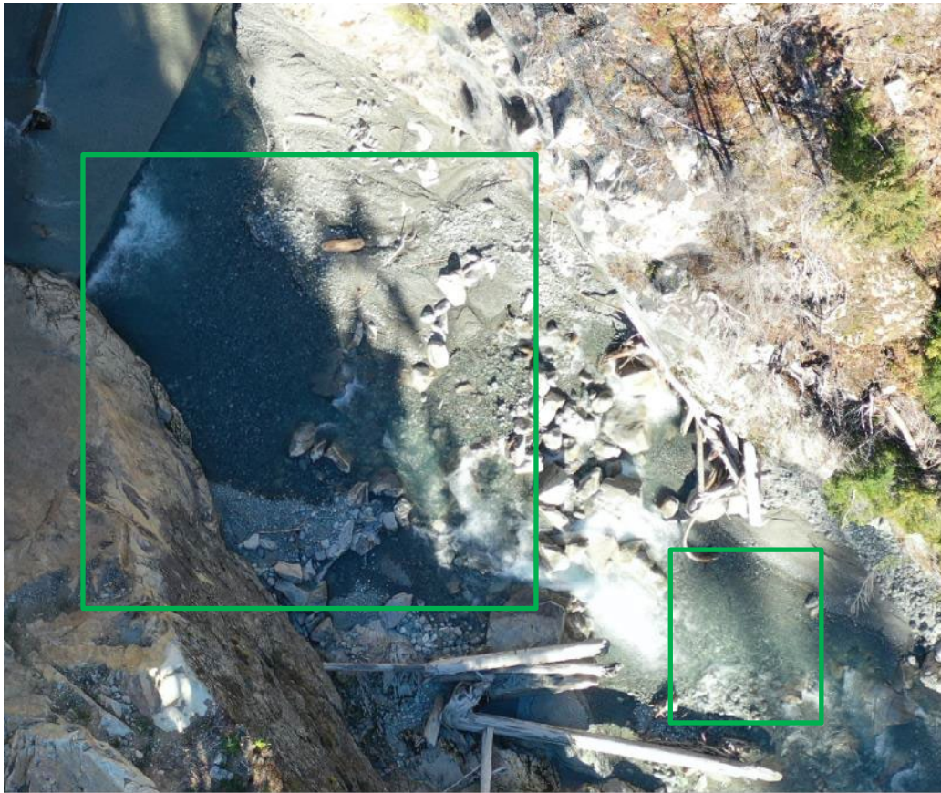
Figure 5. Boulder Creek Diversion Reach displaying gravel deposits outlined in green below the weir captured in 2023 imagery. Evidence of large wood transported through headpond can also be observed. No imagery was collected in 2016 for comparison.
