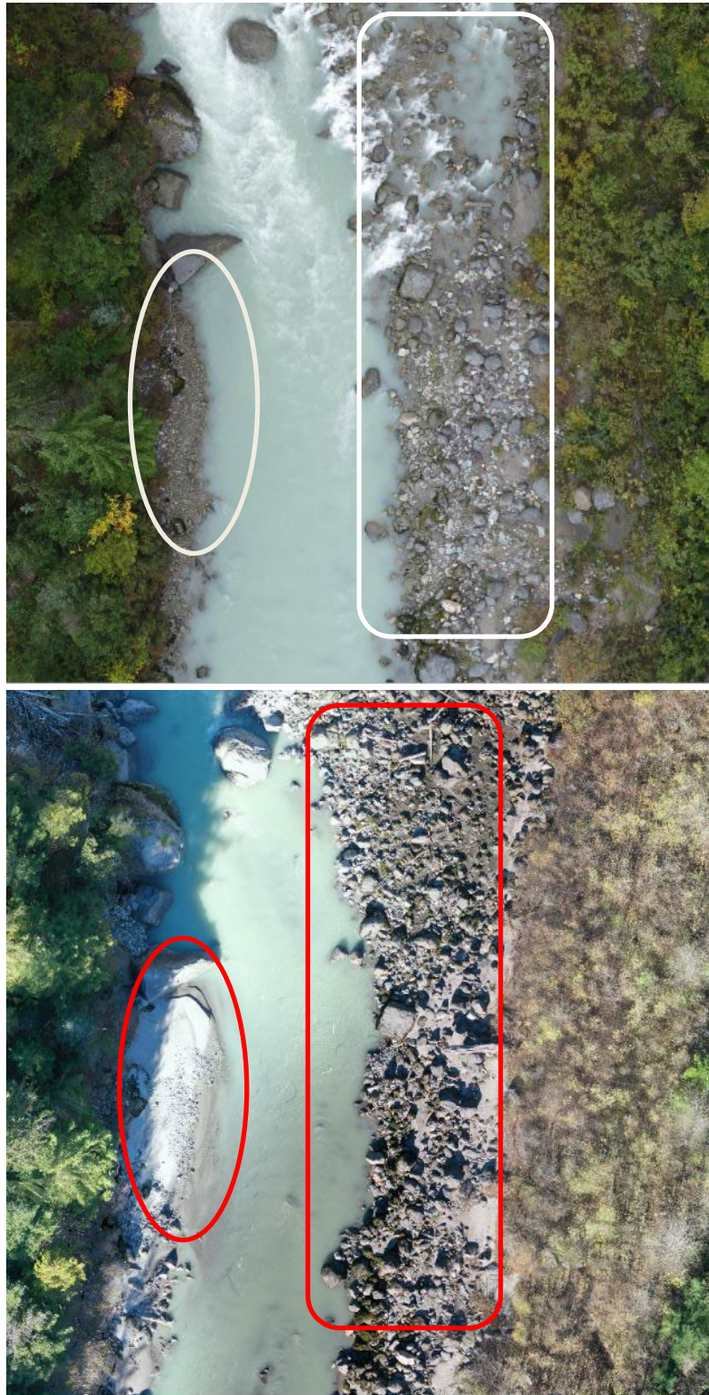
Figure 7. Upper Lillooet River Diversion Reach displaying coarsening of sediment on river left and fine sediment accumulation covering gravel on river right in 2023 (bottom) in comparison to 2016 (top).
