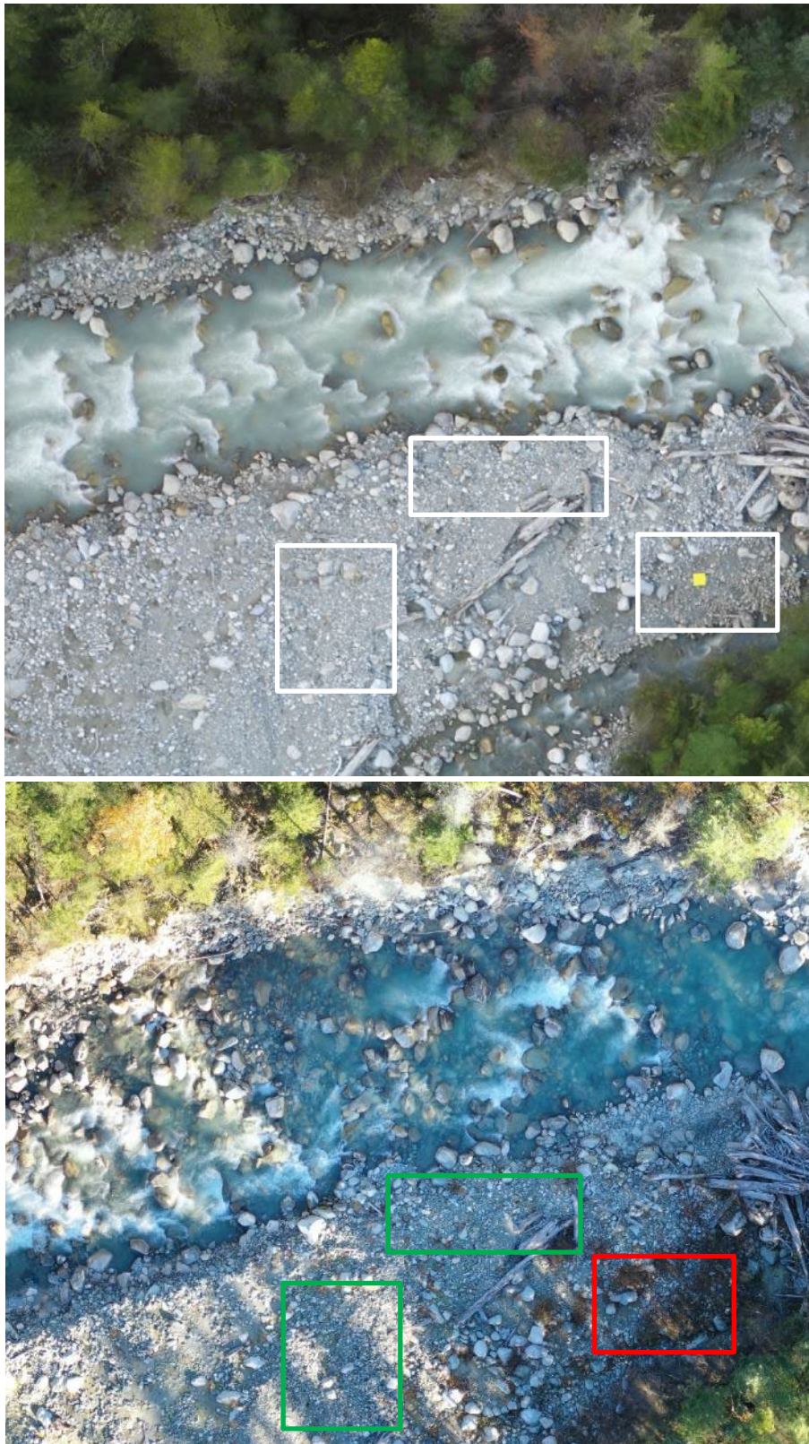
Figure 15. Boulder Creek Downstream Reach displaying both gravel loss outlined in red and gravel gain outlined in green from 2016 (top) to 2023 (bottom).
