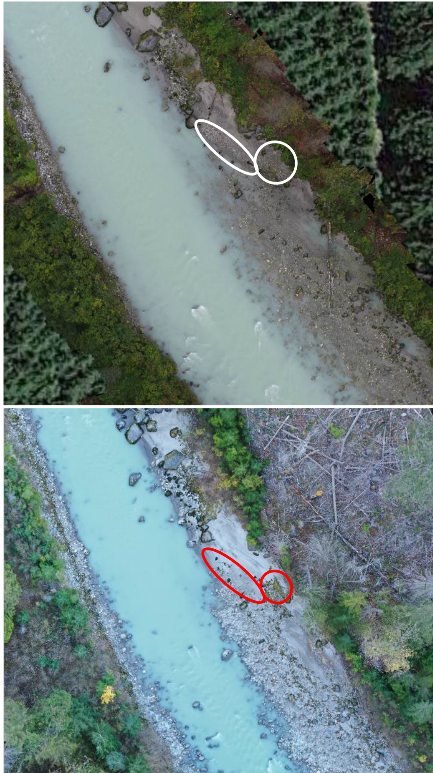
Figure 12. Upper Lillooet River Downstream Reach displaying gravel patches identified in 2016 (top image; orange spray paint) that were covered in fine sediment outlined in red in 2023 (bottom).
