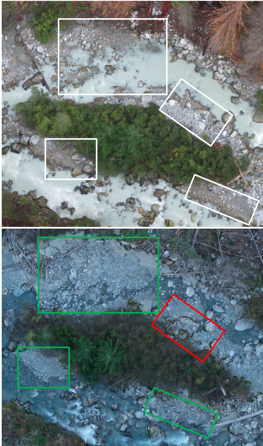
Figure 7. Boulder Creek Diversion Reach displaying gravel accumulation outline in green in most areas and some gravel loss outline in red from 2016 (top) to 2023 (bottom).
