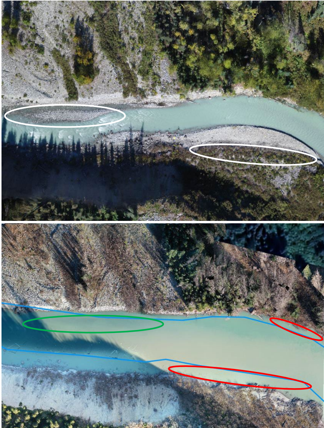
Figure 3. Upper Lillooet River Upstream Reach displaying back watering of channel caused by Upper Lillooet Intake in 2023 (bottom) in comparison to 2016 (top). Blue outline displays 2016 channel path for visual representation. Loss of riparian habitat outline in red on the river left and right bank. Exposed gravel bar outlined in white in 2016 is submerged (green) in 2023.
