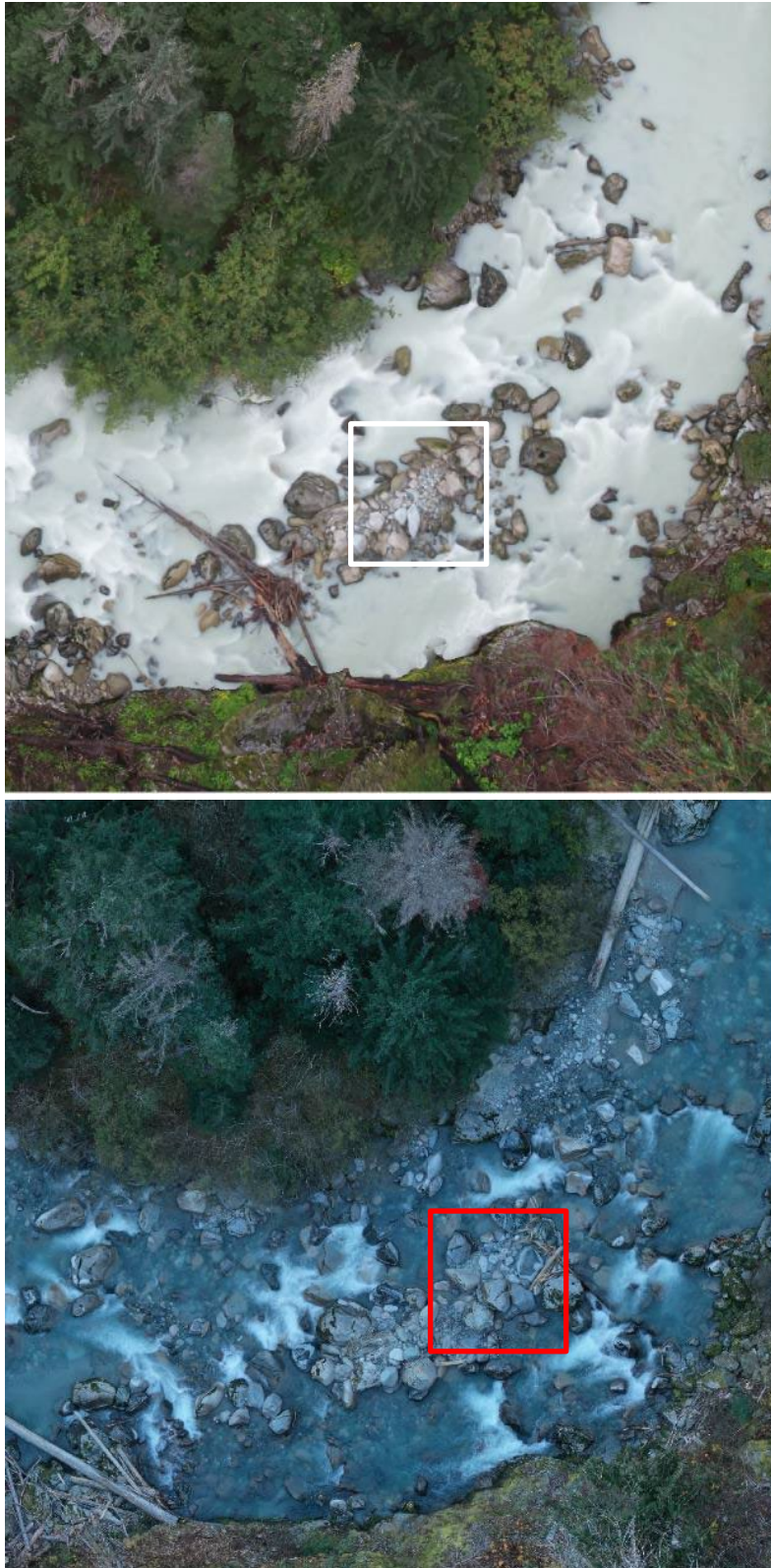
Figure 6. Boulder Creek Diversion Reach displaying scouring of gravel outline in red from 2016 (top) to 2023 (bottom).
