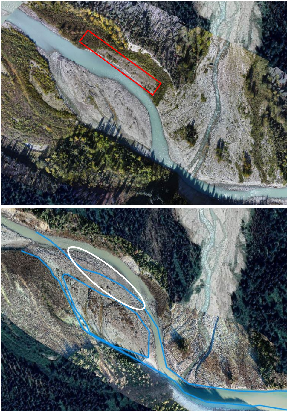
Figure 1. Upper Lillooet River Upstream Reach at the confluence of Salal Creek displaying channel migration towards river left, scouring riparian area outline in red in 2016 (top). Channel migration towards the left bank has caused the mid channel gravel bar to widen outline in white in 2023 (bottom) due to gravel deposition on the right side of the channel cause by slower flows. Blue outline displays 2016 channel path for visual representation of stream morphology changes in 2023.
