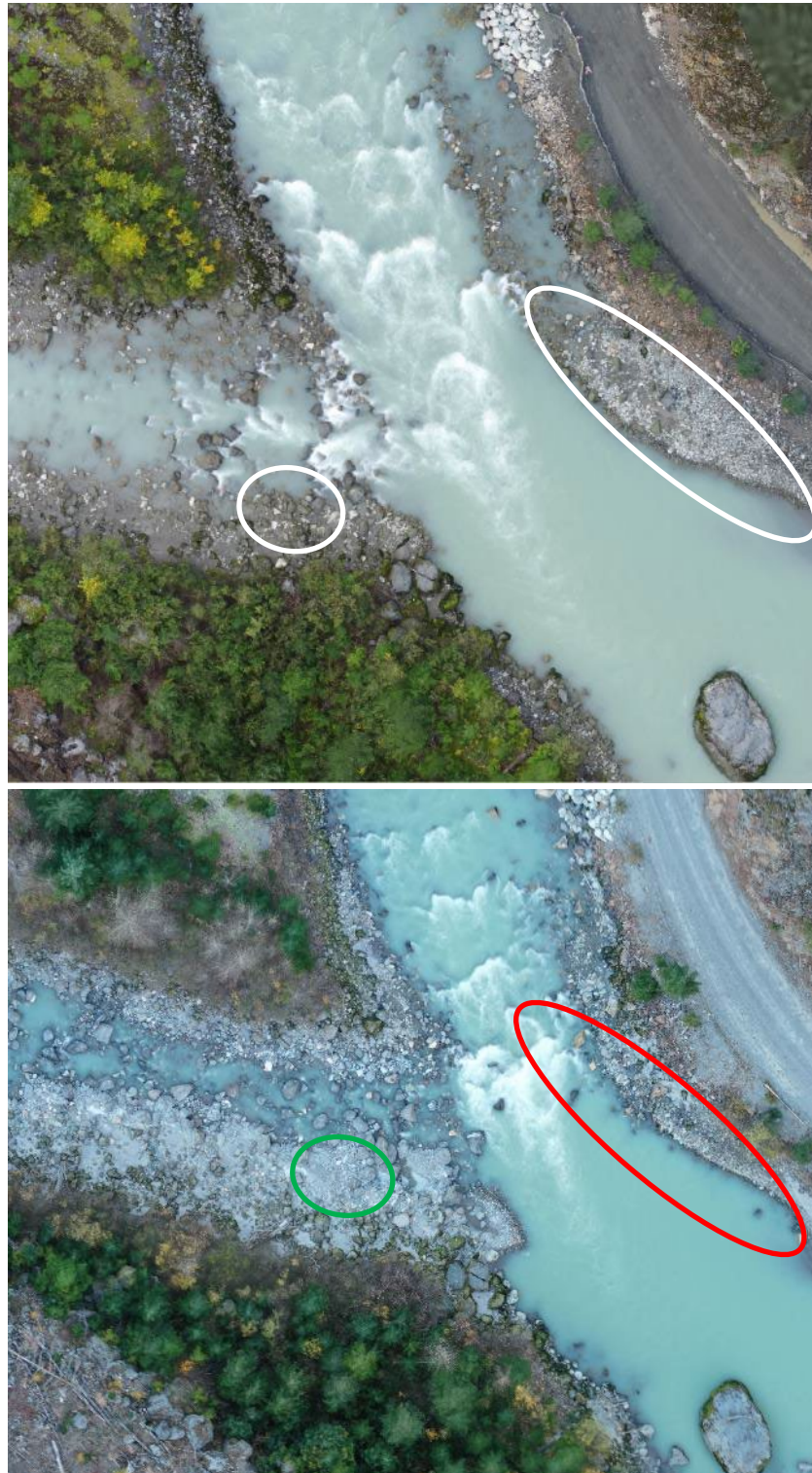
Figure 17. Upper Lillooet River Downstream Reach displaying similar gravel distribution and density in 2023 (bottom) in comparison to 2016 (top). Green outline showing increase in gravel, red outline showing loss in gravel.
