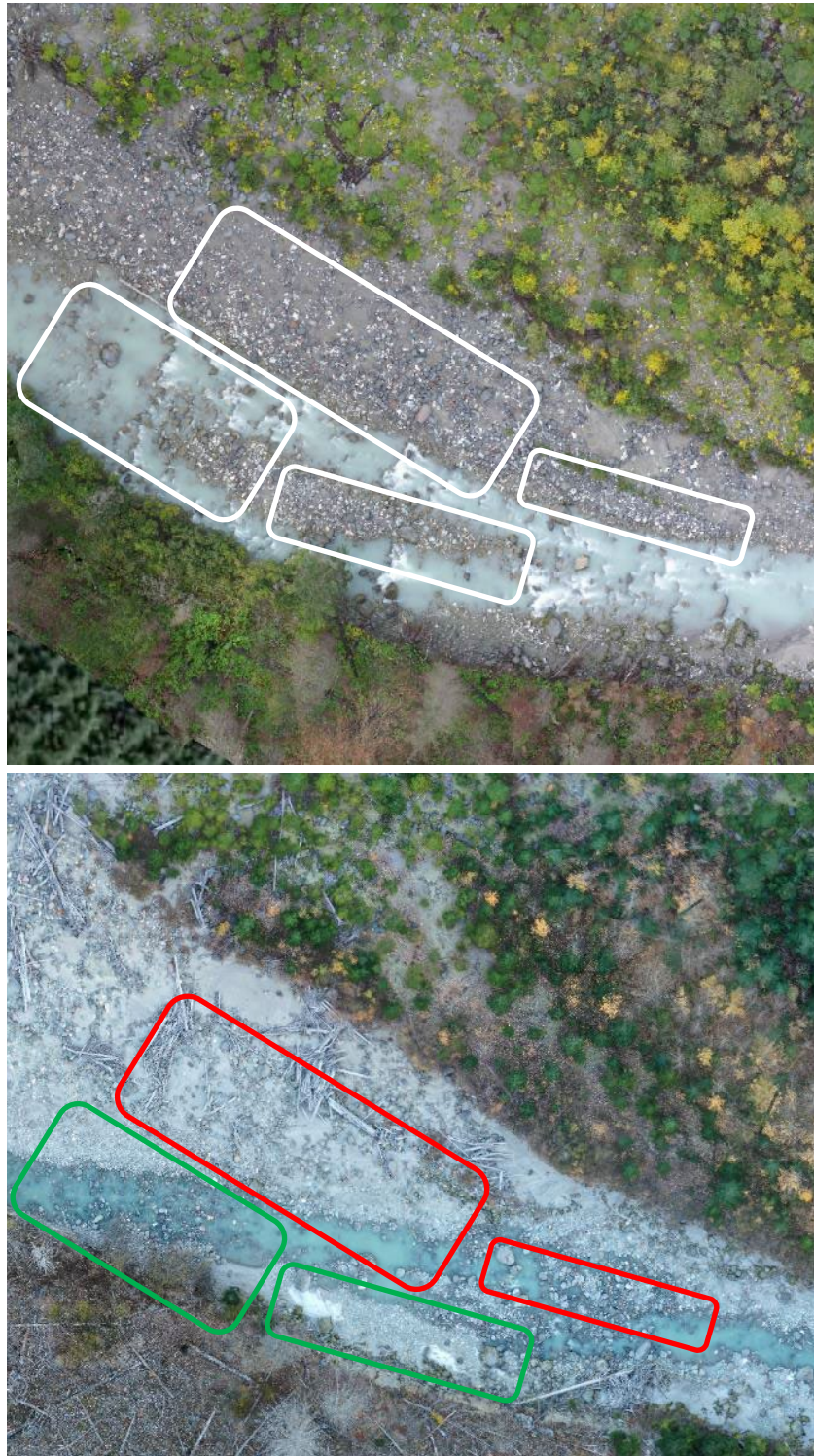
Figure 15. Upper Lillooet River Downstream Reach displaying change in gravel distribution, coarsening, and fine sediment accumulation outlined in red while green outline indicates minimal change from 2023 (bottom) to 2016 (top). Addition of nonfunctional small woody debris likely caused by 2015 firers.
